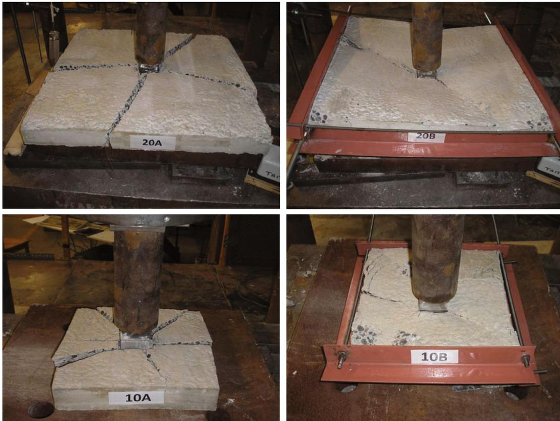
Instead of having a specimen 2B with all edges restrained (confined), two free-edged specimens were tested instead, and labeled as 2A1 and 2A2. Providing edge restraint would have been meaningless, since compressive loading of a fully confined specimen simply causes its material to compress in all directions with artificial strengths increasing, perhaps until such time as the edge members themselves fail.
